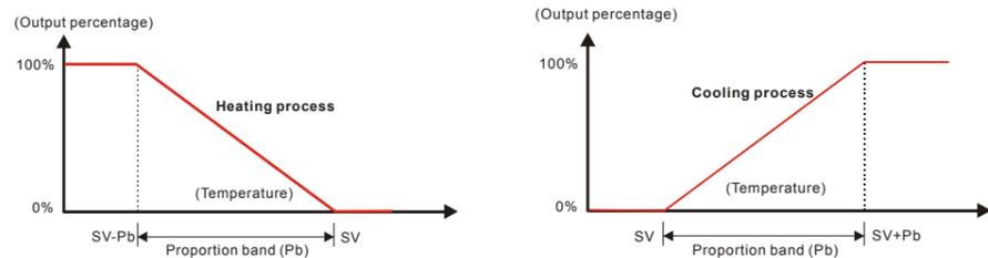
The bigger the parameter P, the less possible that the heating will exceed the SV and the longer it will take for the temperature to reach SV. This is suitable for the control system with faster reaction speed. On the contrary, the smaller the parameter P, the more possible that the heating will exceed the SV and the shorter it will take for the temperature to reach SV; however, unstable control is more likely to occur. Smaller P is suitable for the control system with slower reaction speed.
